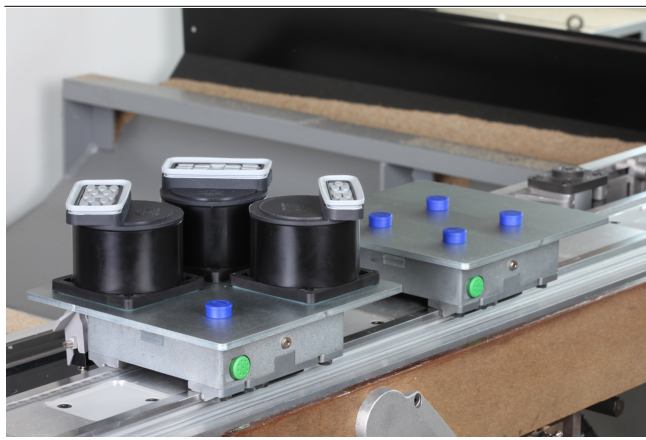
Adapter-Plates ISAP-B with Mono-Base and suction cups for clamping wooden components
